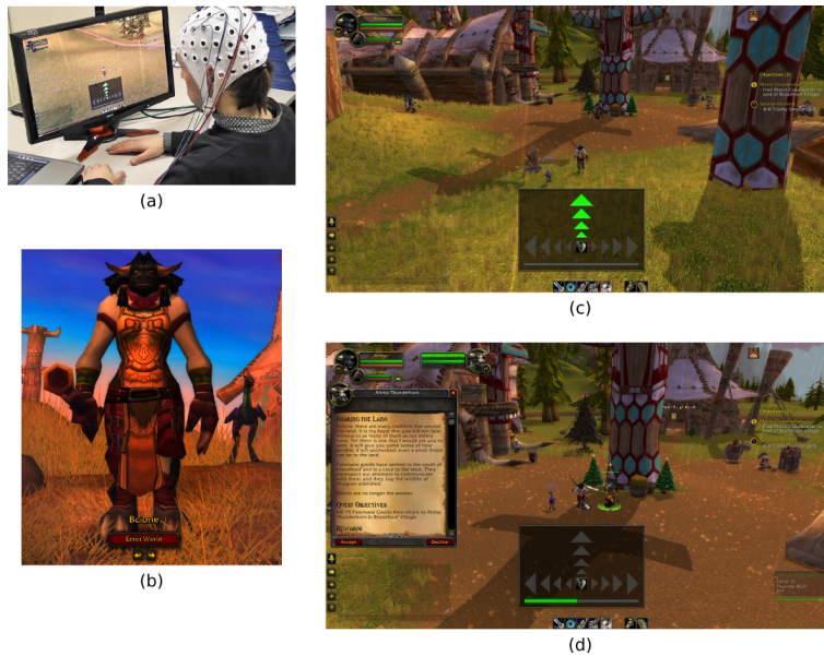
Fig. 2. BCI-based interaction with WoW. (a) Picture of the BCI player in front of the computer screen. (b) Game avatar (level 10 Tauren hunter) (c) The avatar in the starting area Mulgore. At the bottom of the screen, the in-game add-on shows the BCI-operated navigation arrows, and below that, the timeout bar for selecting critical events. In the screenshot, the avatar is walking forward. (d) The avatar is close to a non-playable character that offers him a quest. The timeout bar starts growing from left to right. If the user wants to accept the quest, he has to wait a predefined time. Otherwise, he can move away and cancel the action.
